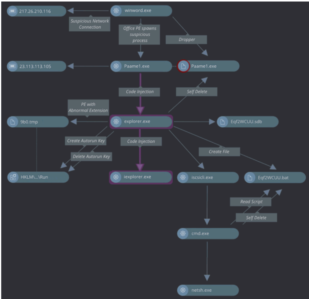
Figure 1 - graph view of Dridex analysis as presented by CyberShield AnD for IT
