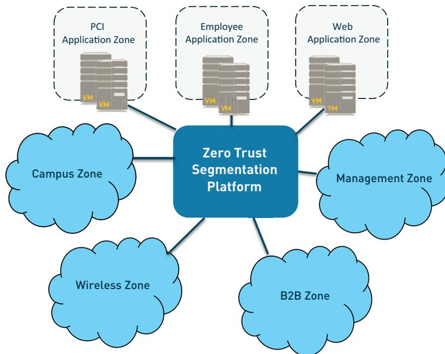
Figure 1 – Zero Trust Conceptual Architecture
